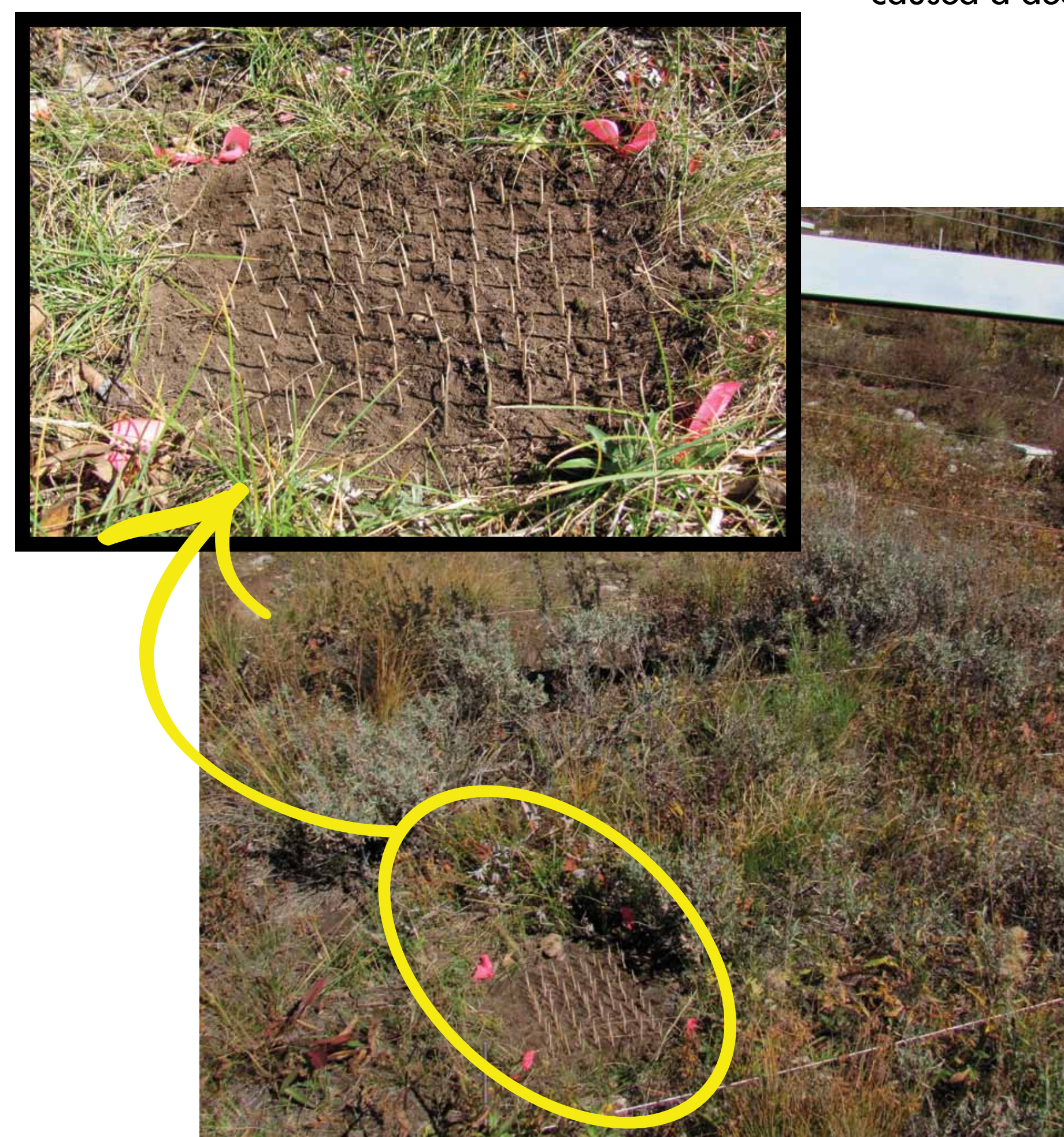
▲ 1. In 1991 we began an experiment to test the effect of global warming on mountain meadows. We suspended infrared heaters above sections of a meadow near Rocky Mountain Biological Laboratory.
