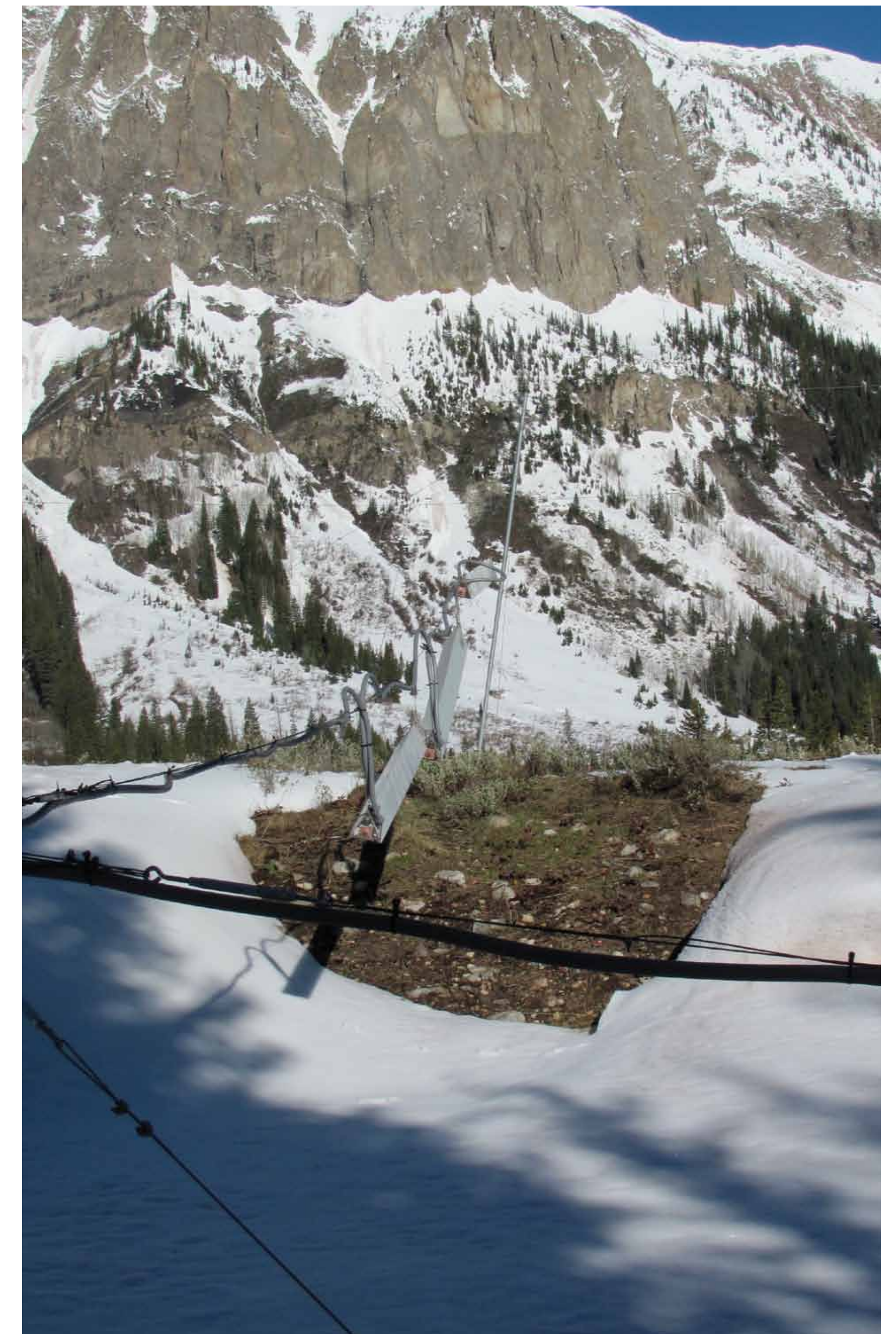
▲ 2. For the past nineteen years, these heaters have caused earlier snowmelt and warmer, drier soils. This experimental warming has caused a decline in the meadow's wildflowers.
