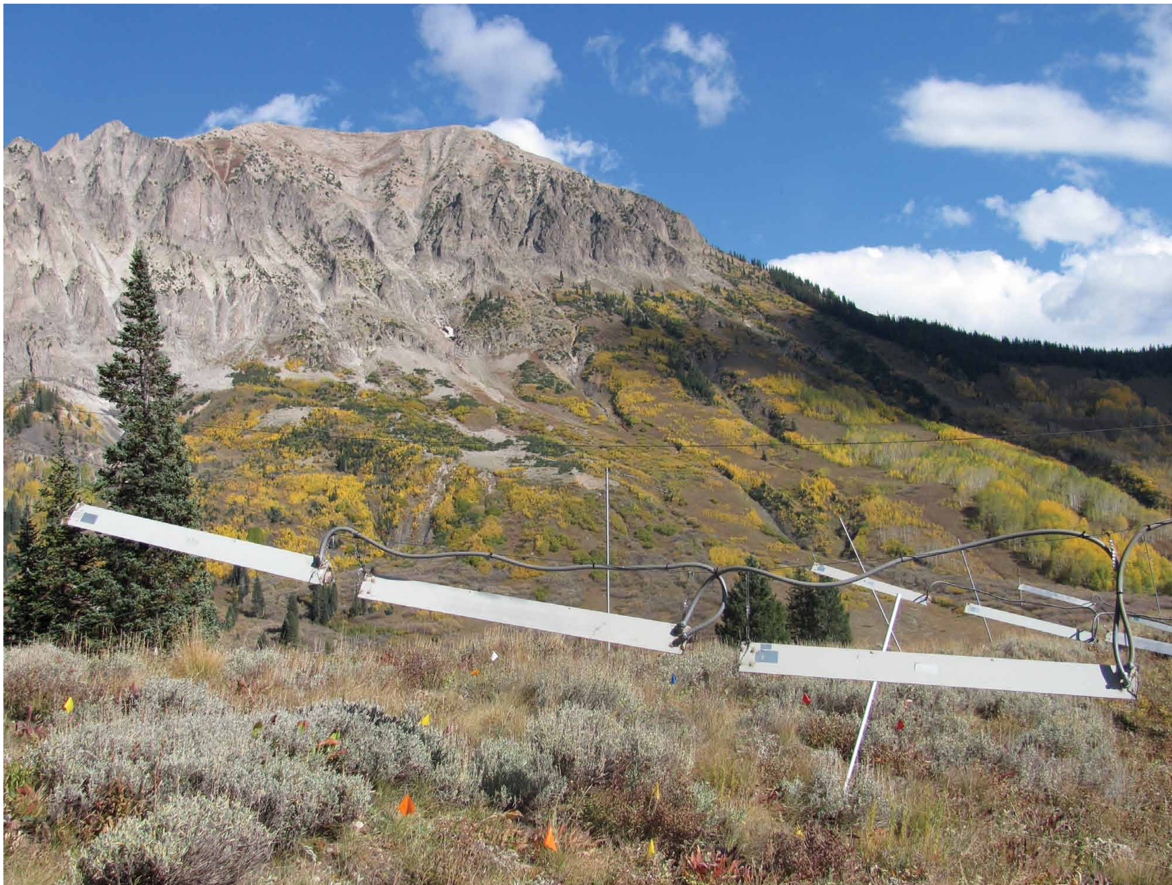
▲ 1. In 1991 we began an experiment to test the effect of global warming on mountain meadows. We suspended infrared heaters above sections of a meadow near Rocky Mountain Biological Laboratory.
