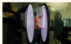
CLTC's laboratory includes state-of-the-art testing equipment, like the integrating sphere (left). A high reflective interior surface measures a luminaire's luminance. An integrating sphere with timed climate control is a new addition to CLTC's equipment.
