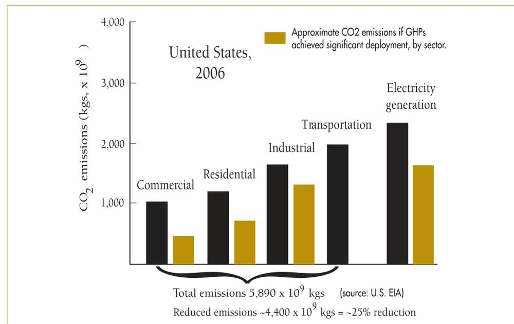
This figure shows the amount of carbon dioxide emitted in the U.S. in 2006, by economic sector. The colored bars show the amount of CO<sub>2</sub> emitted if GHP systems had been extensively used for heating and cooling building spaces in those same sectors
