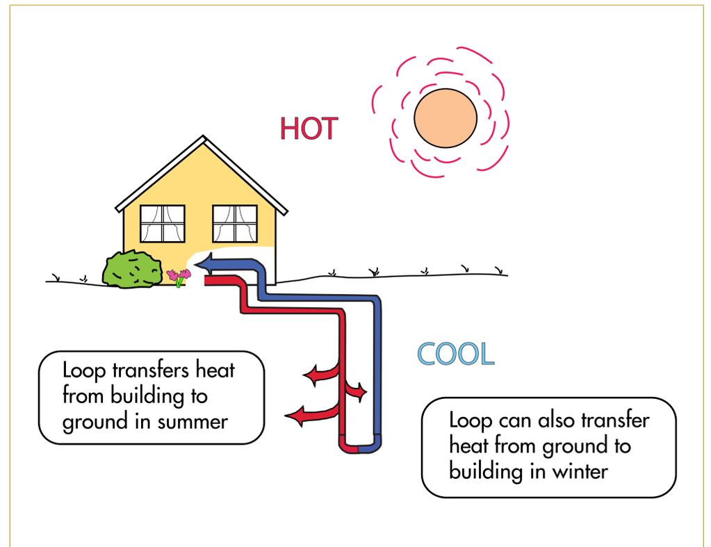
GHP systems circulate a fluid through tubing in the ground. The fluid either obtains heat in the ground and then passes through a heat pump that extracts the heat and distributes it through a building, or removes heat from a building and deposits it in the subsurface. The figure above shows a cooling system for a residence.
