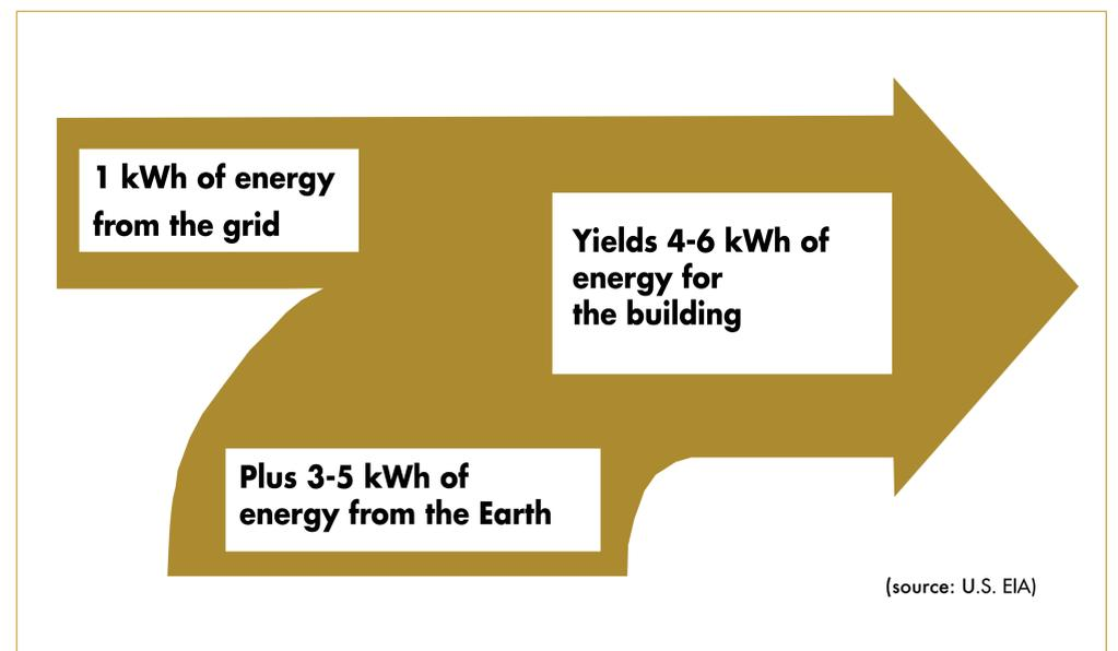
This figure shows the energy sources and resulting output for GHP systems. GHPs provide an efficiency of 400% to 600%. They consume 30% to 60% less energy than typical furnaces with air conditioners. GHPs produce no greenhouse gas emissions; the only emissions associated with them come from the electricity generating technology feeding the grid.
