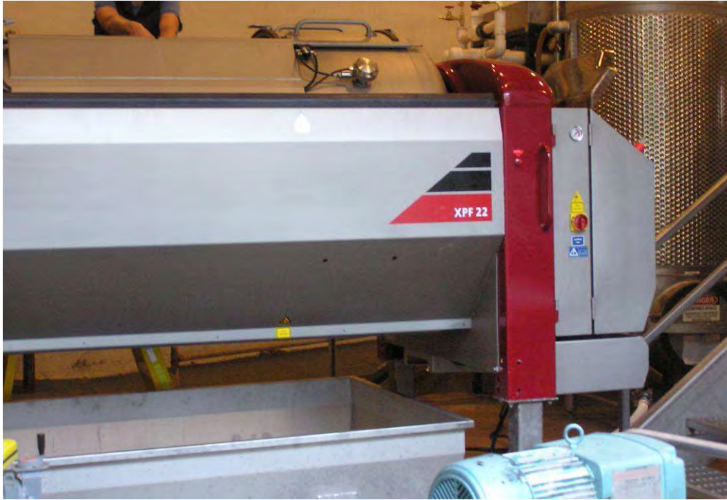
Picture 8 — The 4 x 4 ft bins are placed underneath this piece of equipment and the drum drops directly into the bins.
