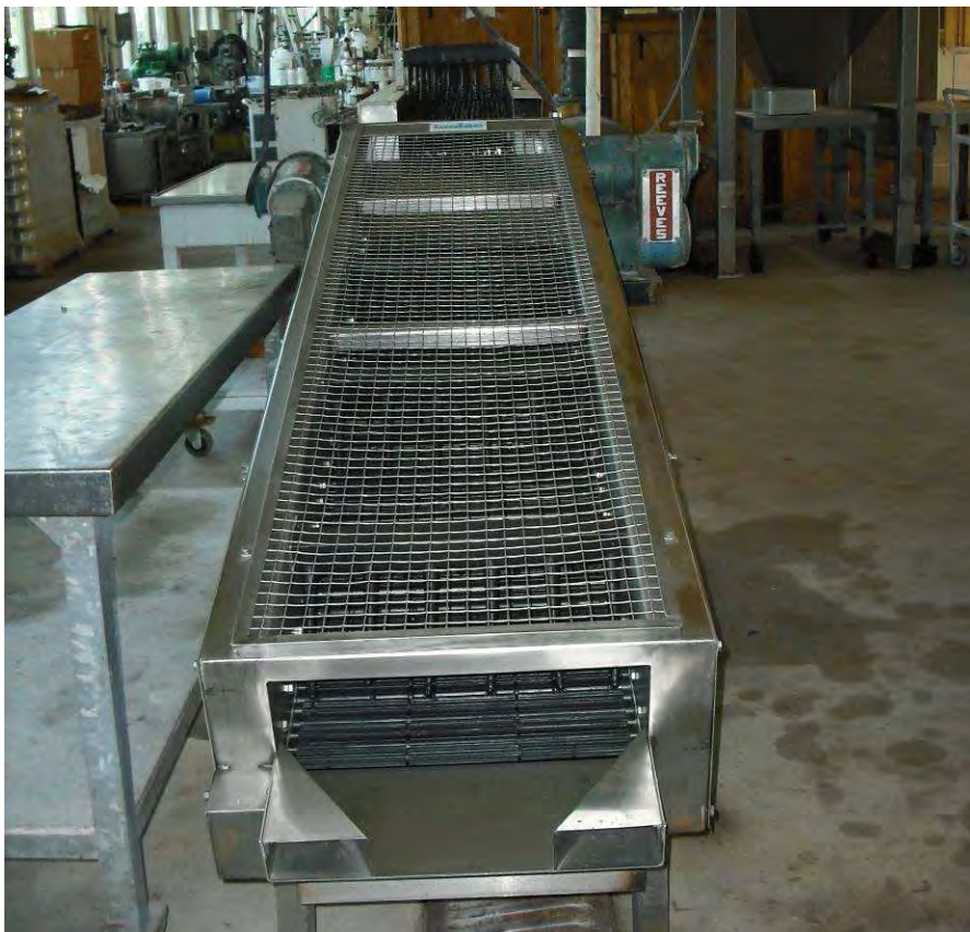
Picture 13 —Peach processing equipment. Where final product is dispensed.
