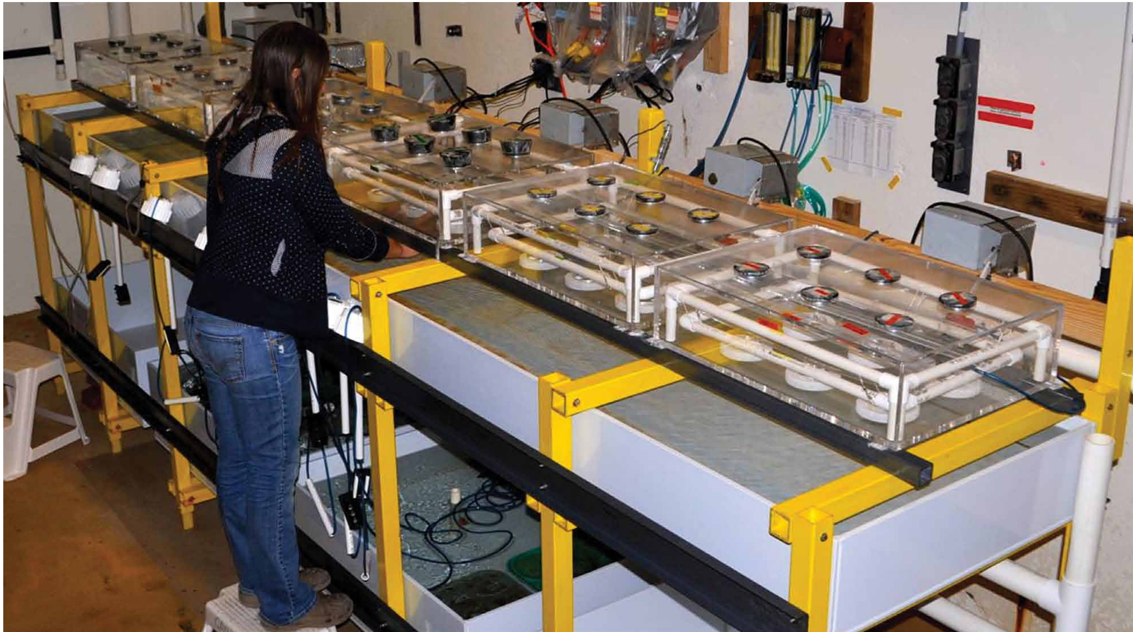
We conducted experiments (above) at Bodega Marine Laboratory to test the impacts of ocean acidification on the growth and survival of native oysters ( Ostrea lurida ). We raised the early life stages of oysters under current atmospheric concentrations (380 ppm) and those predicted by the year 2100 (540–970 ppm). Larval oysters raised in high-CO 2 seawater are smaller (14%) and grow more slowly (38%) as juvenile oysters than oysters raised under today's atmospheric conditions. We are currently investigating whether smaller juvenile oysters experience greater mortality in their natural habitats—an effect that could lead to declines in coastal oyster populations. (Photo: K. Sato)
