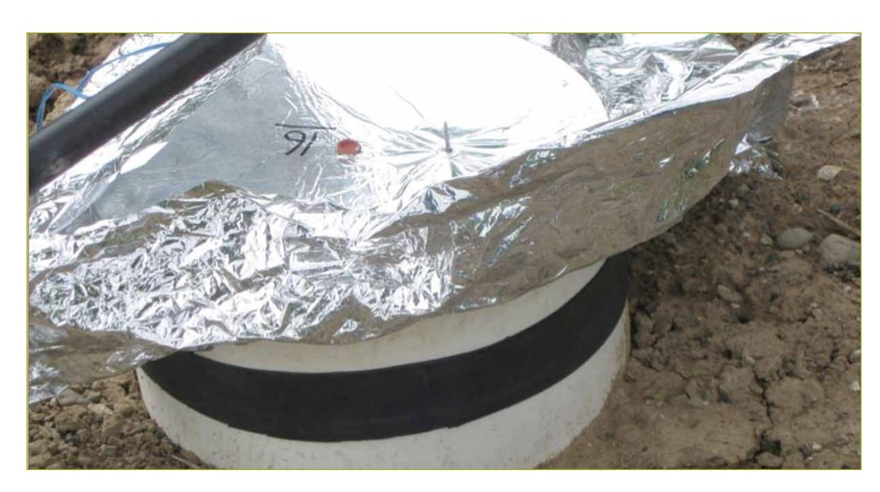
Arr N<sub>2</sub>O emissions are measured using a closed-flux chamber method. The chambers are made of PVC pipe, which is inserted into the ground to a depth of 5 cm.
