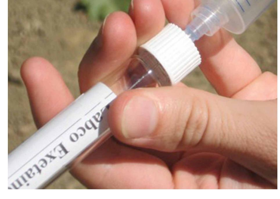
The gas samples are removed from the chambers using an airtight syringe. These samples are then injected into pre-evacuated vials. By measuring the concentration of  $N_2O$  in the vials over three equal time points using a gas chromatograph, the concentration of  $N_2O$  from the soil can be calculated.
