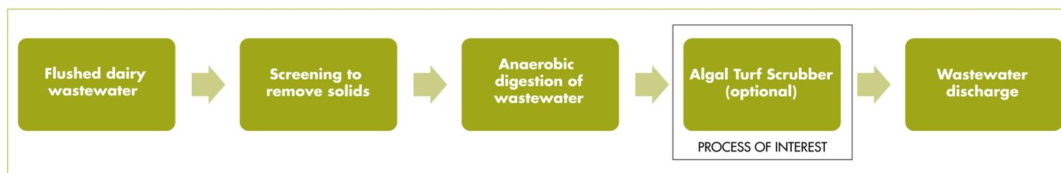
Left is a schematic of the wastewater treatment process. The process was modeled with and without the algal turf scrubber (ATS) in order to understand the impact of ATS on the treatment process. Without the ATS, the treatment process is comparable to existing practice by some dairies in the US.
