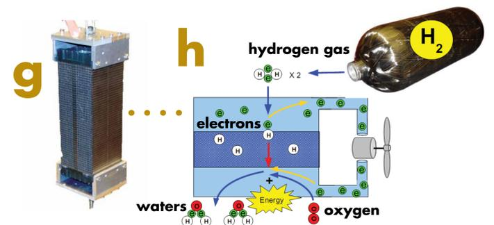
▲ Artificial fuel cells (g) combine substances from a fuel, such as hydrogen gas, with air to produce water and energy (h) much like natural fuel cells. Unlike natural fuel cells, however, artificial fuel cells use rare metals and the proper control of processes within these fuel cells may be problematic.
